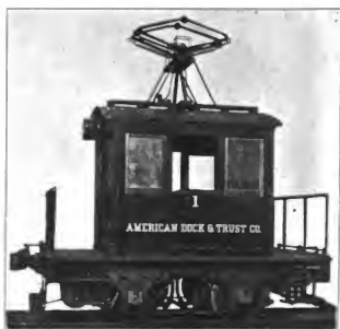
Fig. 4670. Baldwin-Westinghouse Electric Locomotive for the American Dock & Trust Co. Weight, 36,000 lbs.; Wheel Base, 5 ft. 6 in.; Drawbar Pull, Starting, 9,000 lbs.; Drawbar Pull, Running, 6,000 lbs.; No. of Motors, 2.
